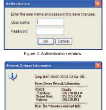
Figure 4. Setup IP Address successfully message.
